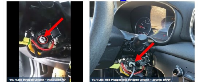
(U//LES) Stripped Column - Milwaukee PD
